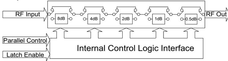
The ZX76-15R5-PN+ parallel interface consists of 5 control bits that select the desired attenuation state, as shown in Table 1: Truth Table
