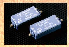
For applications where normal amplifier gain variations as a function of environmental temperature range exceed the allowable system limits. CTT offers amplifier designs whose gain variations have been reduced to one half that of uncompensated designs.
